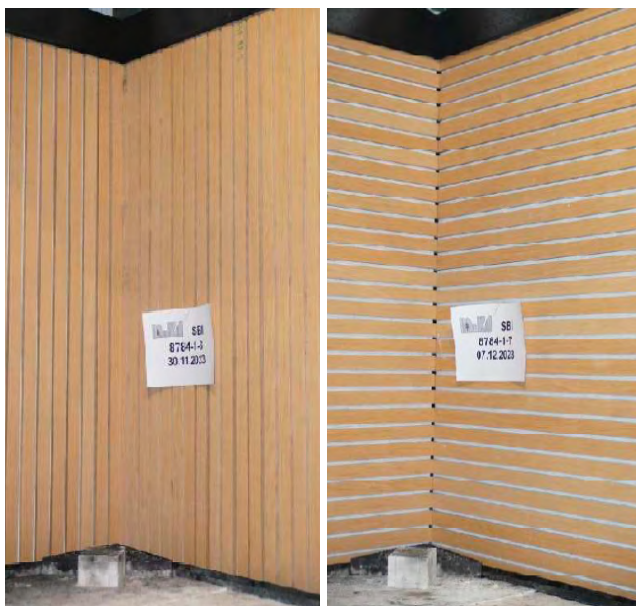
Figure 1: Test assembly at SBI – Vertical and horizontal orientation of slats.
